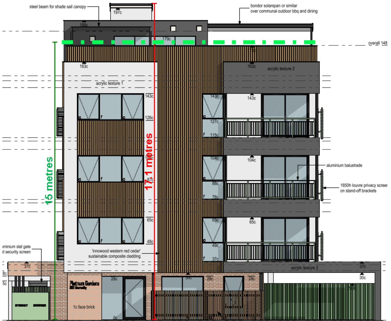
Figure 3: Extract of the street elevation showing the overall building height relative to the 15 metres height limit (dashed green line)
