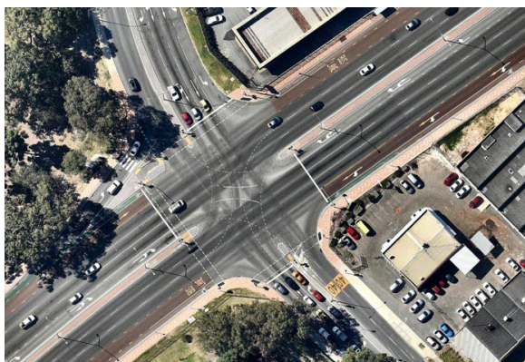
Figure 19 Typical bus lane arrangements at traffic signal intersections along the Great Eastern Highway corridor (source: Nearnmap)
