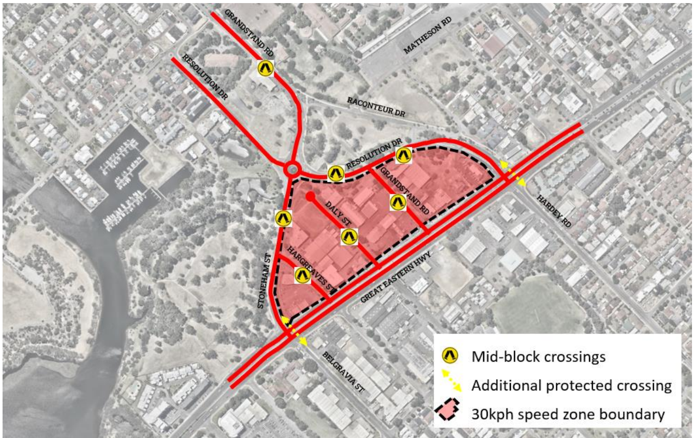
Figure 40 – Recommended Pedestrian and Cyclists Facilities
