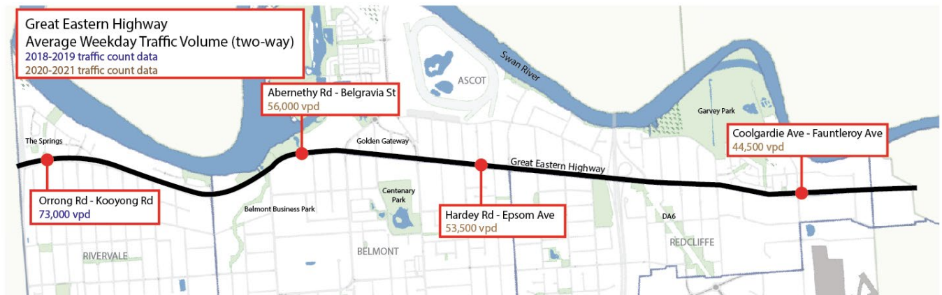
Figure 4 Existing traffic count data – two-way average weekday traffic volumes (source: Main Roads)
